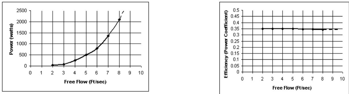
**Fig. 2** Power and Turbine Efficiency versus Water Velocity
