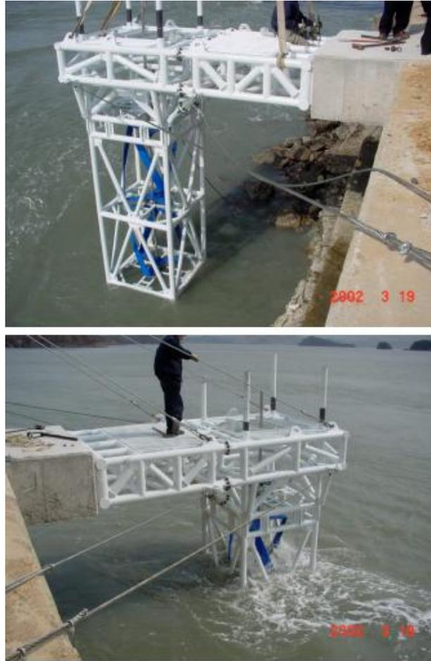
**Fig. 4** Twin Triple-helix Turbine in the Uldolmok Strait (Courtesy of the KORDI Institute)
