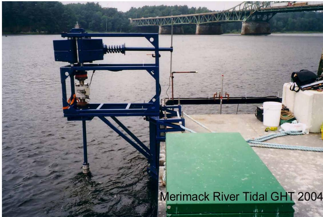
**Fig. 7** Amesbury project. Measurements of turbine and water flow characteristics. The 2.5m height vertical helical turbine sits about 0.5m below the water surface
