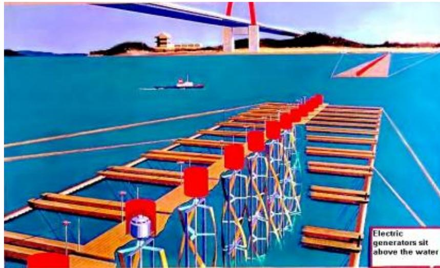
**Fig. 5** Artist rendition of the floating power plant with helical turbines
